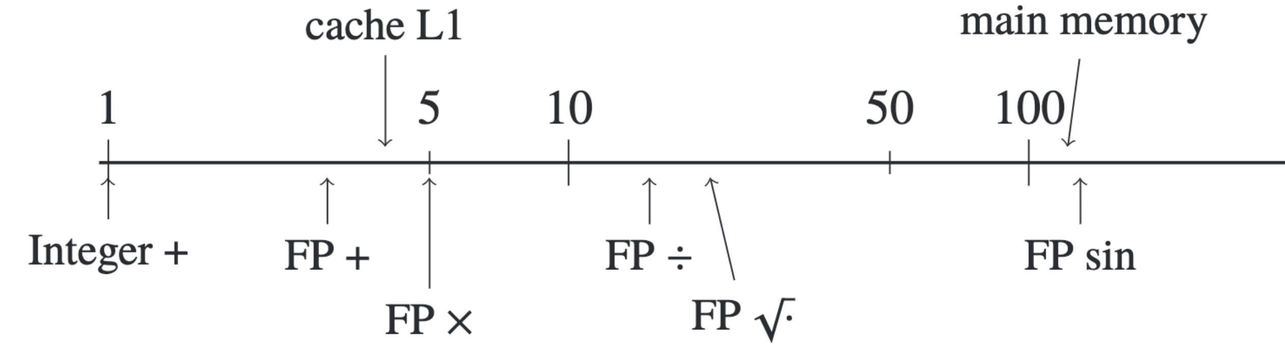
Typical current CPU latencies for FP operations in nb. of cycles (adapted from [1])
