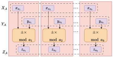
Cons: Division, rounding and modular reduction are difficult to compute in $RNS \Rightarrow$  intermediate operation:Base ExtensionVollmer M., Bigou K., Tisserand A.ARITH-2023, 4-6 September7/24
